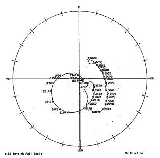
Fig. 1 Polar Plot of the Run before Balancing to Rated Speed, and through to Rated Load.
