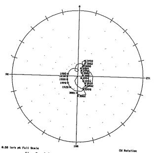
Fig. 5 Polar Plot after Balancing "Critical" Loading, Unloading and Shut Down.
